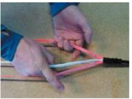
**13.** Now fold the reserve chute with an "S-fold" corresponding to your size and place the rescue container that the rescue flap with the rubber loop looks to the side (seen from the base).
